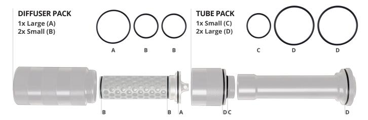
Any loose impurities such as a natural build-up of carbon chips can be shaken out and brushed off where possible. If you wish to further clean the unit, an ultrasonic bath using warm water is adequate. DO NOT use any harsh chemicals they may damage the moderator. Afterward, allow parts to dry fully before re-assembly. A light coat of a water displacement oil can be used. You may clean threads and use a little grease to help lubricate and protect them.
